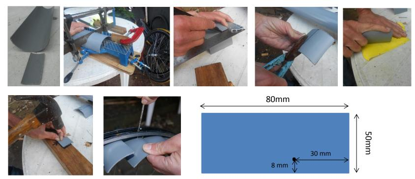
Clearance holes for the screws need to be drilled through the rim of the wheel 8mm in front of each spoke. 36 vanes are required so it is useful to use jigs to ensure uniformity. A starter hole for the fixing screw is best made with a nail – but only make a deep mark in the surface. The vanes are set asymmetrically to give clearance to the belt or rope. The can be symmetrical if using a chain with a large cassette.
