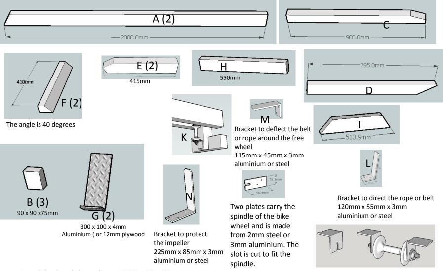
Seat roller and pulley units (4). The dimensions of the brackets will vary with the bicycle wheel hubs used. My thanks to Jack Owako in Kenya for this idea.
