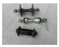
Front wheel hubs are needed for the seat rollers and pulleys but note that a matching pair is needed for the seat
