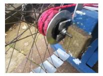
If using a rope, a large washer needs to be fitted to the freewheel unit. The size and fitting will vary with the unit used.
