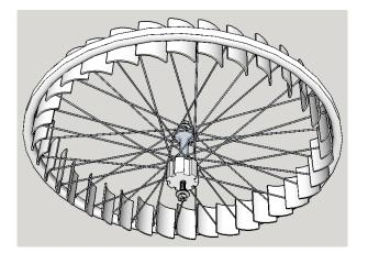
This impeller is more efficient and easier to make than the one used in previous models. The vanes are made from plastic guttering and held in place with self-tapping screws. Note the direction of rotation – which is clockwise as seen from this side
