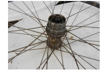
The freewheel unit screws on to the wheel. This unit is 'stepped'. The straight ones are better
