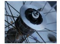
Most freewheel systems have a threaded collar to hold the sprockets in place.. This can be used to secure the washer.
