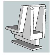
The dimensions of the seat need to be determined by the athletes using the machine. The lower plate is screwed to the main part to clamp the seat in the required position.
