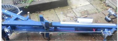
The handle return action using a bicycle inner tube. The last piece of rope adjusts the tension
