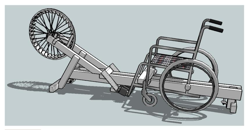
This is the additional component required (shown with the latches open) to fix the wheelchair in position. The dimensions need to fit the particular wheelchair but as a guide it will be about 410mm long. The centre of the wheelchair needs to be in line with the chain/rope/belt.
