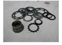
The freewheel unit with sprockets removed – specialist tools are needed
