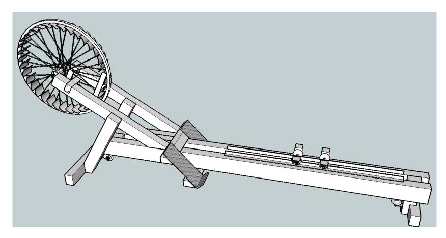
This has a re-designed impeller that is more efficient and easier to make, also it can adapted to use either a belt or rope drive. The seat is not shown in order to be able to see the rollers.
